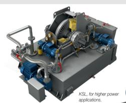
In addition, Transfluid says the system: eliminates the stationary element, the scoop, and hydrodynamic resistance in the working circuit; operates in forward and reverse; and has all key accessories mounted externally.
