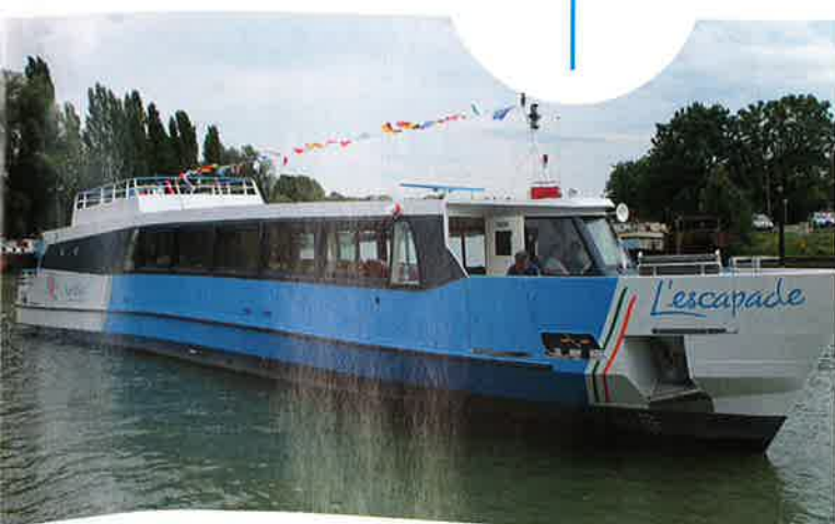
3. Alumarine's L'escapade passenger vessel, operating in France, is equipped with a Transfluid hybrid system
