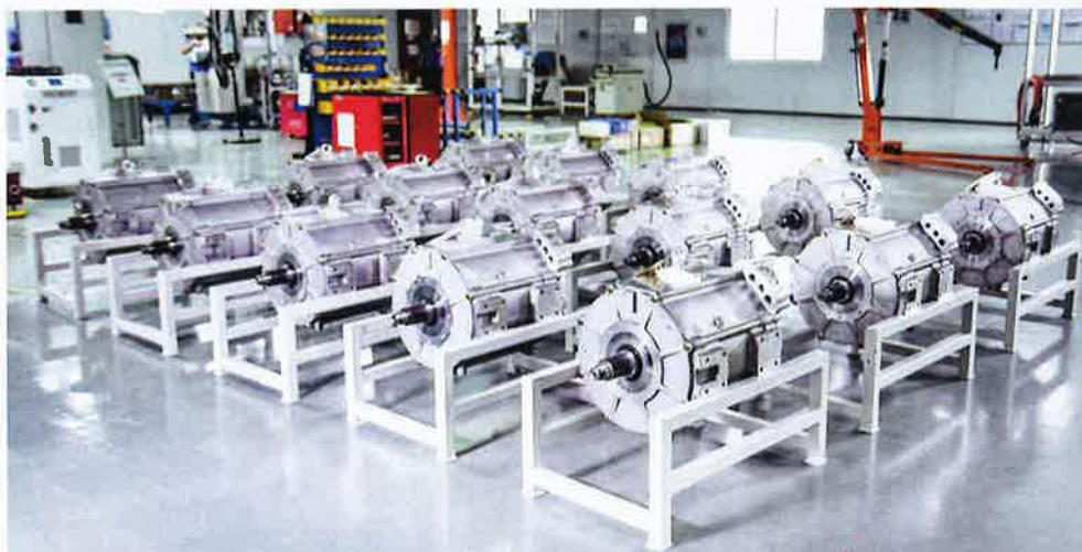
TM4 SUMO systems interface directly with standard rear differentials of medium- and heavy-duty vehicles.
