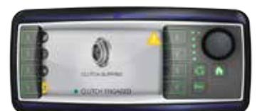
Warning and alarm messages are sent via CAN BUS to the operating machines PLC or Transfluid Display.
