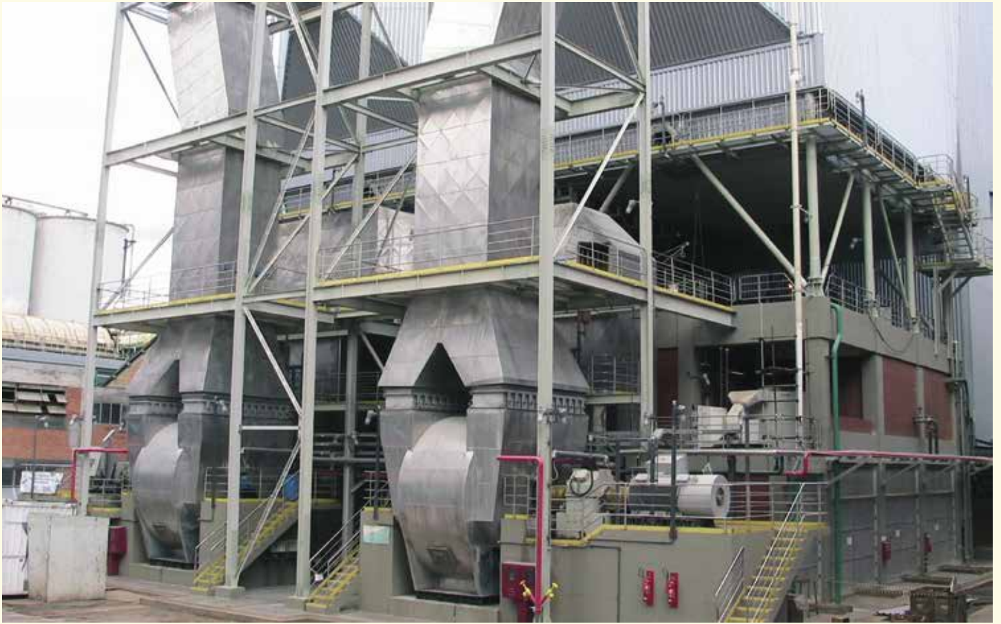
2xD34 KSL, 2000 kW - 1200 rpm, Fan drive (Brazil)
