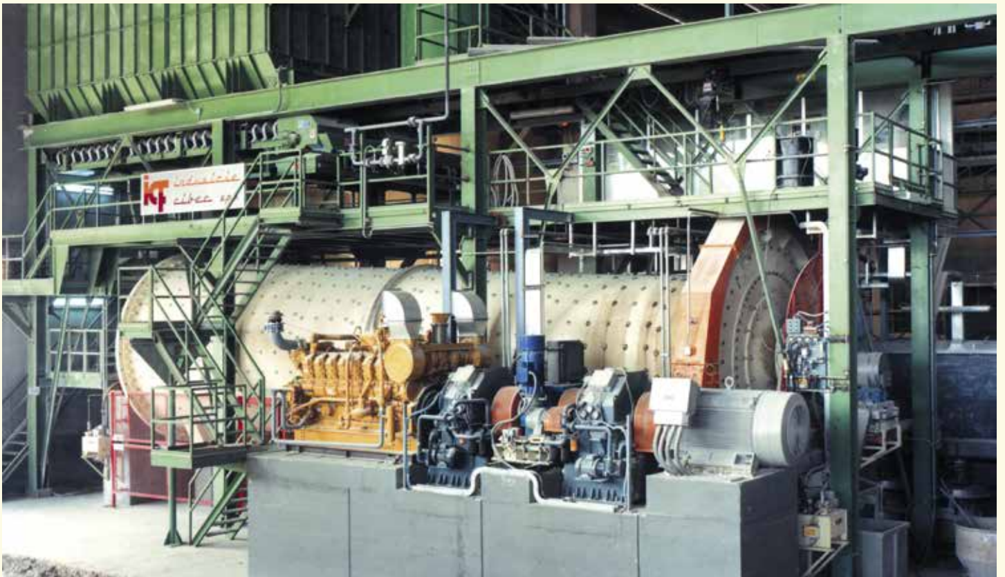
2x34 KSL, 630 kW - 1000 rpm, Ceramic mill (Italy)
